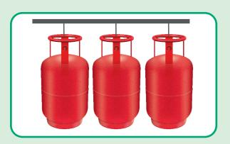
Always keep cylinder connected to manifold.
