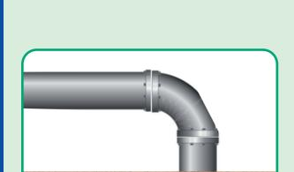
Always install LPG pipeline above ground level.
