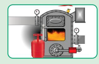
Never store or use LPG cylinders near chimney, boiler or furnace.
